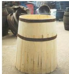
Barrel under construction
